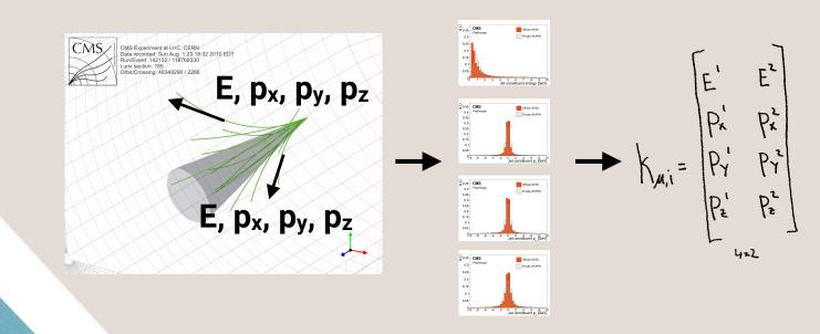
Ensures network can 1) learn the sum of momenta in the jet 2) learn the momenta of each constituent 3) make linear combinations of particles during training (e.g for W $\rightarrow$ qq, w<sub>4,1</sub> = w<sub>4,2</sub> because (k<sub>µ,1</sub>+k<sub>µ,2</sub>)<sup>2</sup> = M<sub>W</sub><sup>2</sup>. Allows network to "groom" away unimportant particles).
